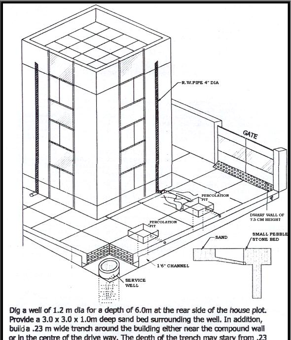
or in the centre of the drive way. The depth of the trench may stary from .23 m near the gate(entrance) and run through 0.45 m at the rear end of the plot towards the well. The trench has to be connected to the deep sand bed constructed around the open well.
